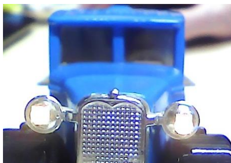
The three photos above show the LEDs off (left), then at about 5 milliamps (middle), then overwhelming at full brightness, 20 milliamps (right). It may look better with round LEDs and may be converted in the future.
