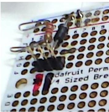
The two photos above show the connector board that will be mounted under the platform or perhaps in the foam. The resistor is shown on the left with long leads so that it may be changed easily for different light levels.
