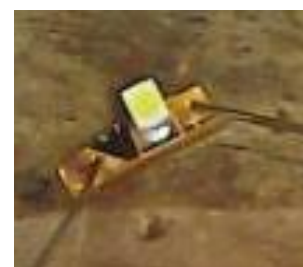
Figure 12 – De-solder the other side
