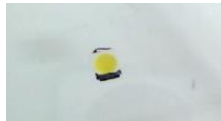
Figure 18 – LED marked black on cathode side
