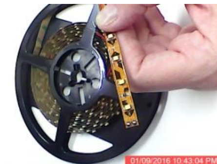
← Figure 6 - Different style removed from package showing lead in. These are not waterproof, but are easier to work with.
