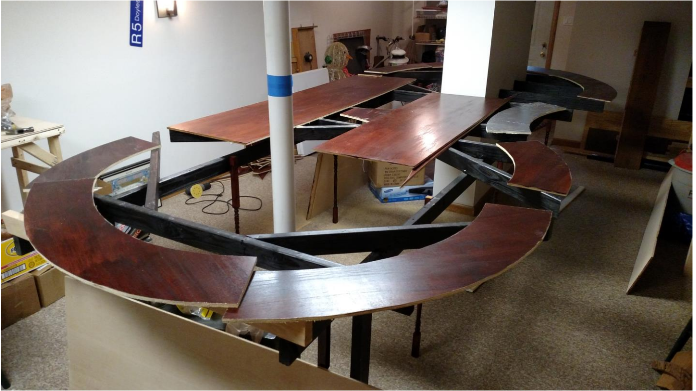
Ron's finished subroadbed is ready for splice plates and final positioning
