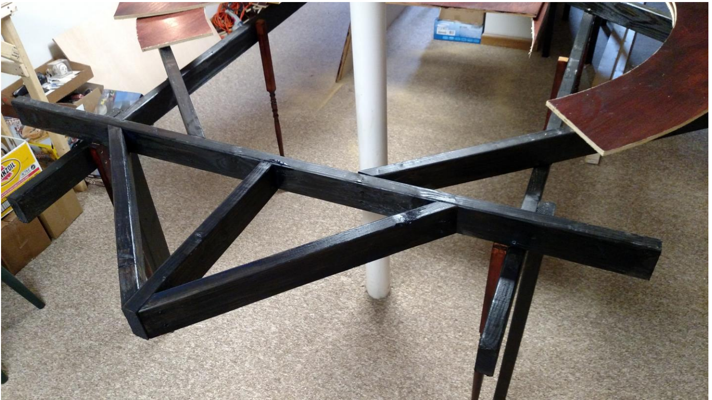
Ron's substructure was cut and assembled from his CAD plan to exactly match the subroadbed. Phase 2 will include a second level portraying Cassandra on the PRR Middle Division main line. The second level will extend the layout into the adjoining room.
