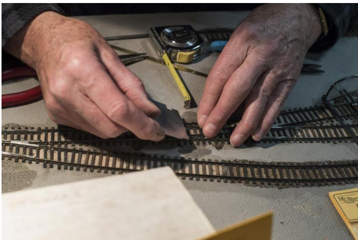
Charlie Woodward checks flangeways with an NMRA gauge
