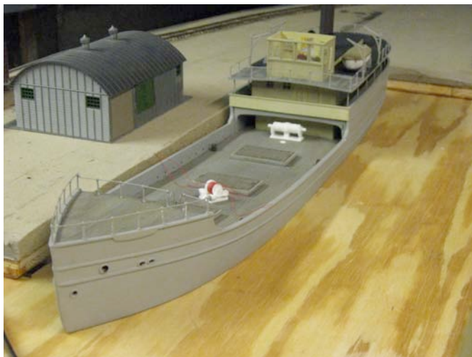
This bow shot shows the cut down bow, handrails, cargo deck area, and in the background the new bridge structure.
